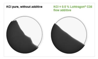
**Proven Flow Functionality by Funnel Testing** Your requirements regarding vertical flow properties of Lohtragon<sup>®</sup> C36 are tested by using a stainlesssteel funnel. This method is performed according to Ph.Eur. (2.9.16) under defined conditions.
